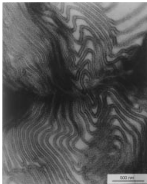
Figure 5. Transmission electron micrograph of S_{27}B_{15}C_{58}^{219} isothermally crystallized at 42 °C (stained with OsO_4 ).
